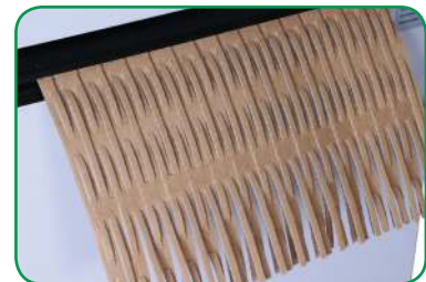
Produces flexible perforated cardboard netting, at speeds of up to 40 fpm
